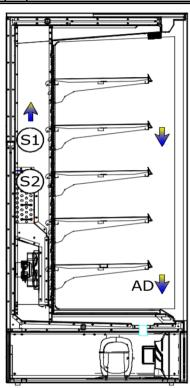
1 - LOCALIZATION OF CONTROL PROBE 2 - LOCALIZATION OF DEFROSTING PROBE, DEFROSTING HEATERS
