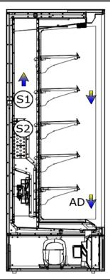
1 - LOCALIZATION OF CONTROL PROBE 2 - LOCALIZATION OF DEFROSTING PROBE, DEFROSTING HEATERS
